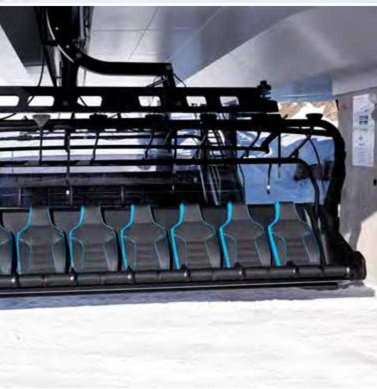
The new D-Line 8-seater chairlift "Visnitzbahn N2" acts as a feeder to the Alp Bella sector of the ski area in Samnaun. With a capacity of 3,500 passengers an hour, it impressively fulfills its purpose. Equipment features include seat heating, bubbles and a locking system that keeps the restraining bars locked during the trip. The mesh banners on the backs of the chairs tell the story of the village and ski resort Samnaun in striking images.
